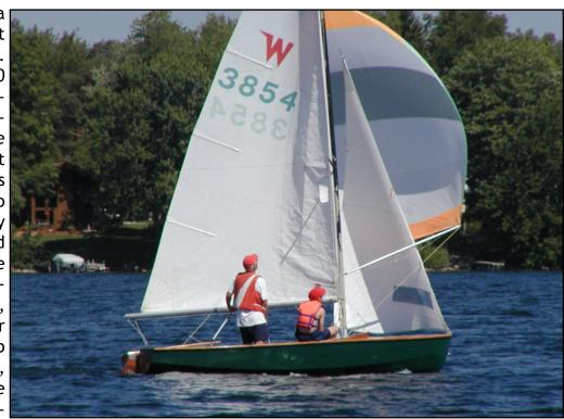
ported by the boom. A small outboard motor can be fitted, and it's easy to lower the mast - even single-handed - to pass under bridges.
